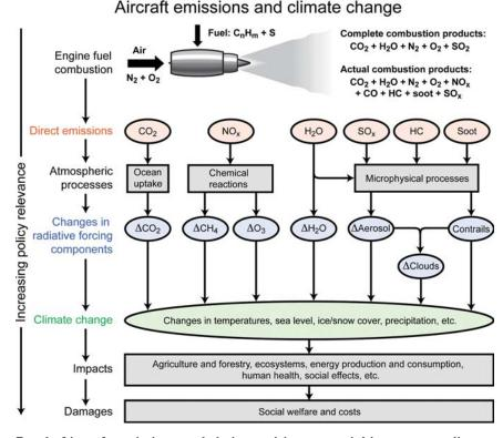
FIG. 1. Aircraft emissions and their resulting potential impacts on climate change and welfare (developed for a special report for the International Civil Aviation Organization, but adapted from Wuebbles et al. 2007; based on Penner et al. 1999; Fuglestvedt et al. 2003).
